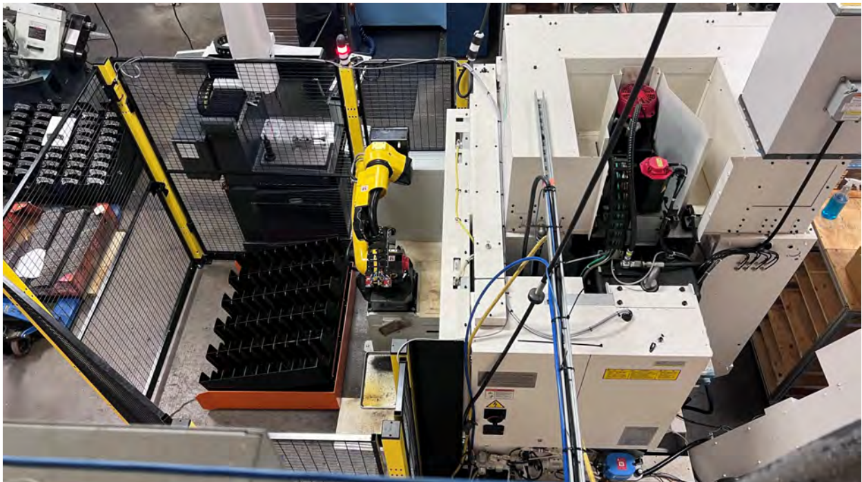
Bird's eye view of Fanuc Robodrill, Robotic cell and CMM
