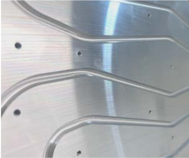
Cooling Plate - Interior
