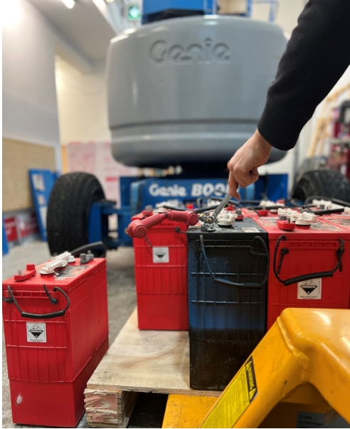
Original led acid batteries being removed from genie lift.
