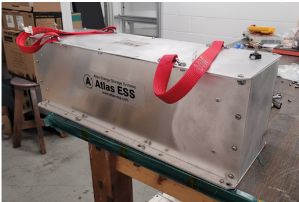
An Atlas ESS enclosure configured to fit the battery bay in the genie lift.
