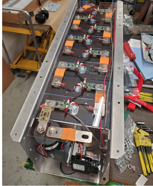
Battery back during assembly process using lithium-ion phosphate modules with a total of 7.2 kWh capacity.
