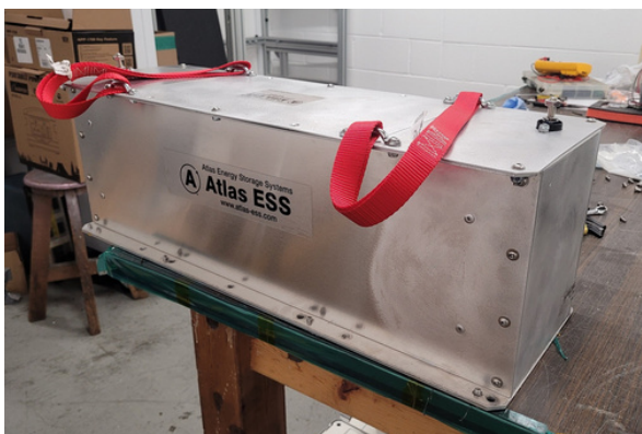
An Atlas ESS enclosure configured to fit the battery bay in the Genie-Telescopic boom lift.
