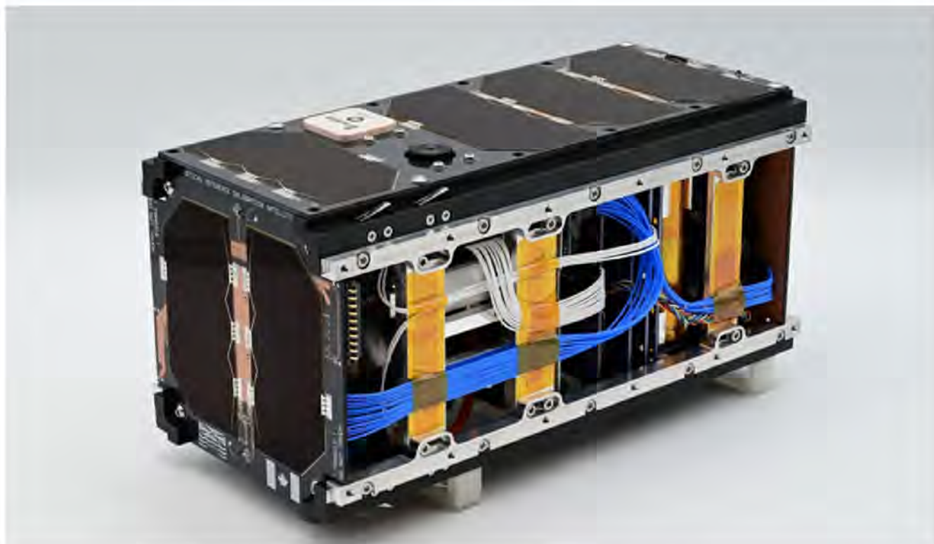
Final assembly of the spacecraft with a solar panel removed.
