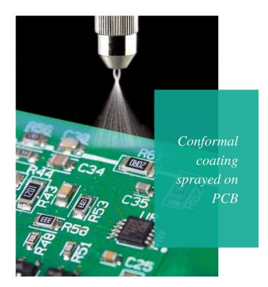
automated or semi-automatic, and can accommodate a wide range of component sizes and shapes. They are designed to provide a precise and consistent application of the coating material, ensuring that all areas of the electronic components are adequately covered. They are commonly used in various industries such as aerospace, automotive, consumer electronics, and medical devices, where the reliability and longevity of electronic components is critical.
